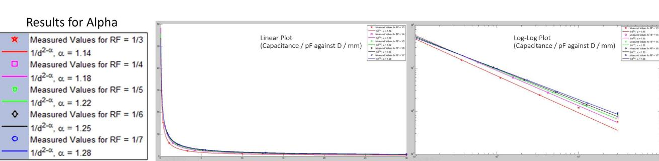
RESULTS: Alpha values increase with the denominator of removal factor as theory predicts. Howevr, all alpha values are > 1. Possible explanations: fringing effects due to finite area parallel plates, the imprecise thickness of dielectric layers due to resolution limits of 3D printing, the presence of stray capacitance from other sources, and also the higher sensitivity to changes in smaller pF values in log plot.
