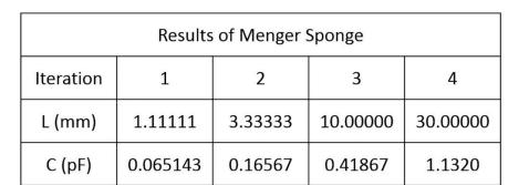
1V to GND was applied across the dielectric. Scaling was accurate, but not best-fit. Curve had to be amplified by factor of 1.2 for best fit line with the scatter plot.
